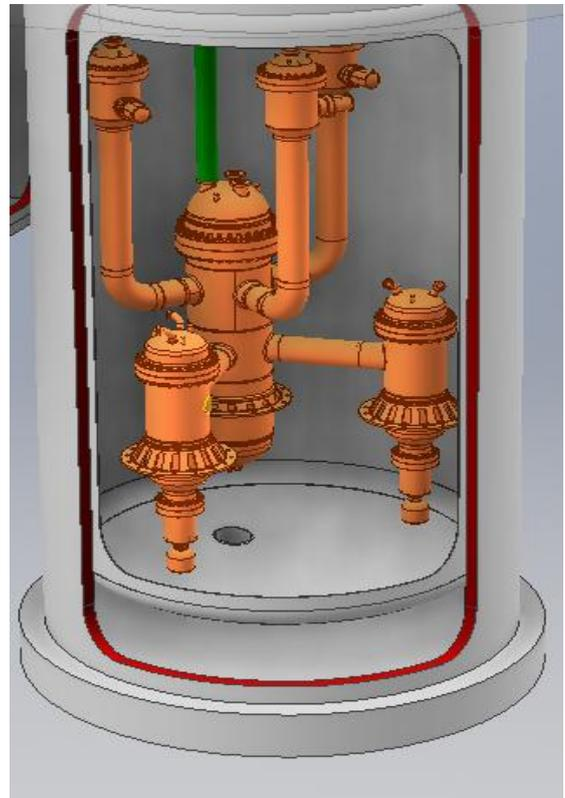
The original design of the ALLEGRO consists of two He primary circuits, three decay heat removal (DHR) loops integrated in a pressurized cylindrical guard vessel. The two secondary gas circuits are connected to gas-air heat exchangers.
